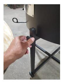
To install the optional wood shelf loosen the top bolt with knob and allow leg to fold down. Place shelf on bottom cross bars and reassemble the leg. The barrel can also fit in this lower area for more compact storage. Be a sure the barrel is cool with no fire before placing in this area.
