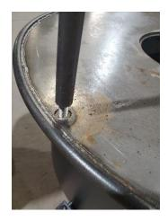
Screw the vertical post in the hole of the flat cook top. Tighten nut with lock washer below the flat cook top. Post should be firm and not wobble if properly tighten.
