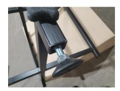
Assemble adjustable feet or caster wheels to the bottom of the legs in the threaded metal caps.
