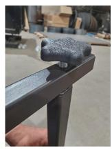
Two of the bolts have knobs for quick disassembly. First assemble legs to cross bars using these bolts with knobs.
