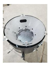
Install fire basket with tabs supporting itself on the rim of the barrel. Set flat cook top on the rim of the barrel keeping the overlap evenly spaced around the entire circumference.
